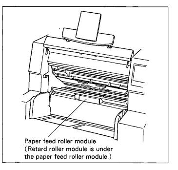
Use the accessory roller cleaning paper to wipe off the dirt on the surfaces of the paper feed roller and separator roller.
